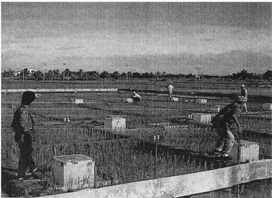
Figure 2-5 Gas collection chambers in experimental plots
