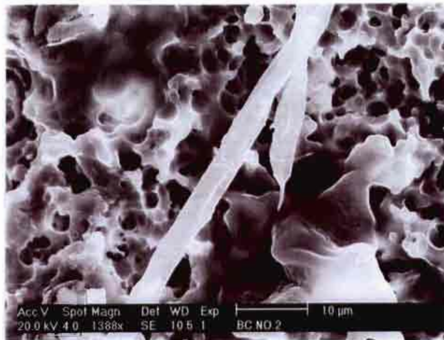
Figure 9: Scanning electron micrograph (1388x) of the IPS-Empress bar subjected to a slow cooling in air.
