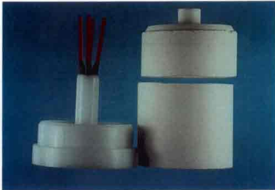
Figure 1: Resin patterns were sprued (left) and then invested with a phosphate bonded investment mold as per lost-wax technique. Mold sectioned in half.
