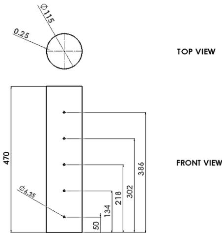
Fig. 2: Core of the biochar kiln (dimension displayed in millimeters)
