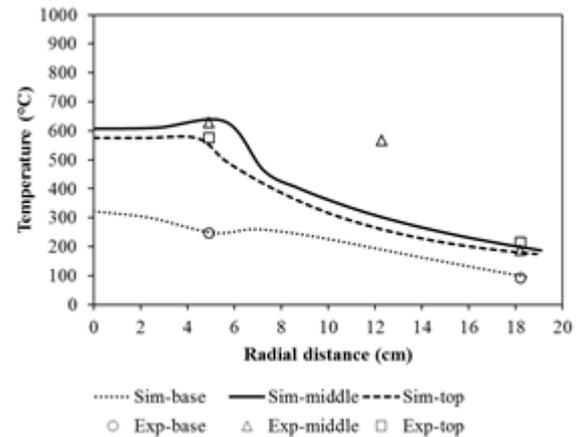
Fig. 4: Temperature simulation compared with experiment along radial direction in biochar kiln at base ( $h_1 = 80$  mm), middle ( $h_2 = 261$  mm), and top ( $h_3 = 385$  mm) of the kiln with corncob as feedstock
