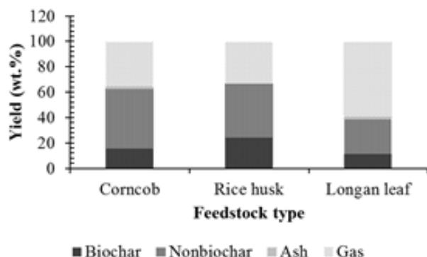
Fig. 10: The weight percent of yields for each feedstock type
