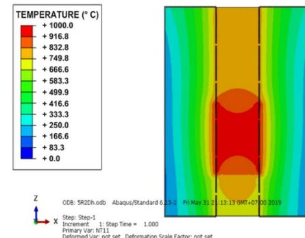
**Fig. 9:** Temperature distribution in biochar kiln with dry longan leaf as feedstock
