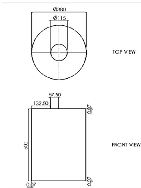
Fig. 1: Biochar kiln (dimension displayed in millimeters)
