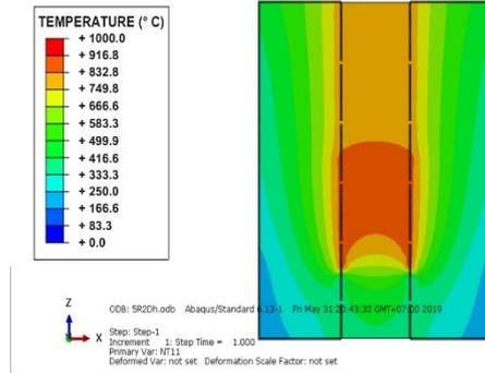
**Fig. 7:** Temperature distribution in biochar kiln with corn cob as feedstock
