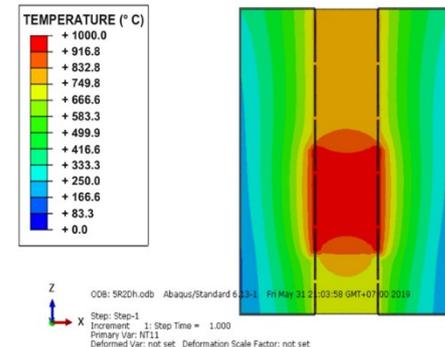
**Fig. 8:** Temperature distribution in biochar kiln with rice husk as feedstock
