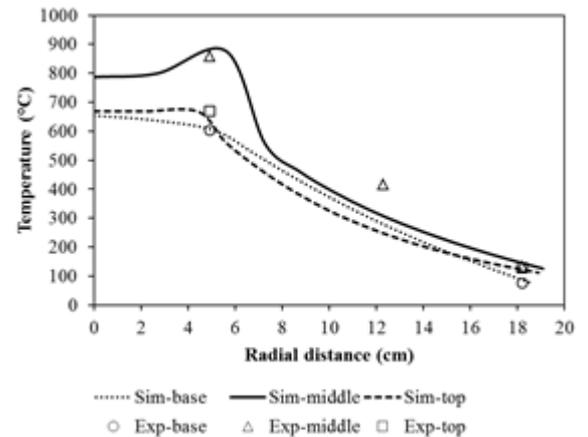
Fig. 5: Temperature simulation compared with experiment along radial direction in biochar kiln at base ( $h_1 = 80$  mm), middle ( $h_2 = 261$  mm), and top ( $h_3 = 385$  mm) of the kiln with rice husk as feedstock
