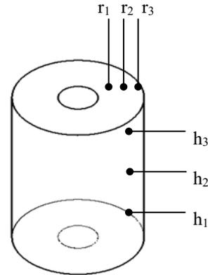
Fig. 3. Thermocouple attachment at different longitudinal and radial positions ( $h_1 = 80$  mm,  $h_2 = 261$  mm,  $h_3 = 385$  mm,  $r_1 = 49$  mm,  $r_2 = 123$  mm, and  $r_3 = 182$  mm)
