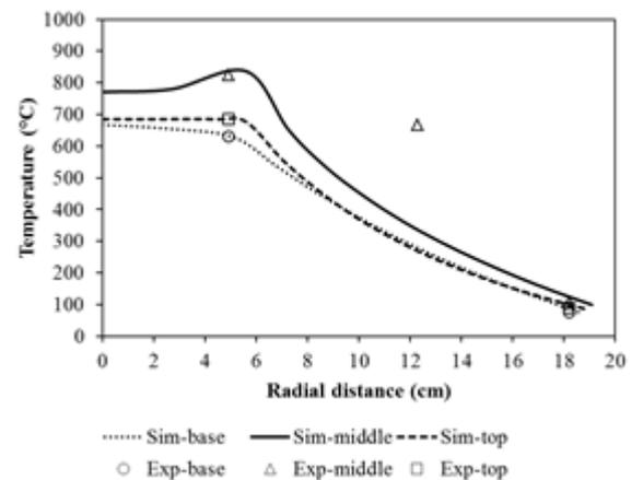
Fig. 6: Temperature simulation compared with experiment along radial direction in biochar kiln at base ( $h_1 = 80$  mm), middle ( $h_2 = 261$  mm), and top ( $h_3 = 385$  mm) of the kiln with dry longan leaf as feedstock
