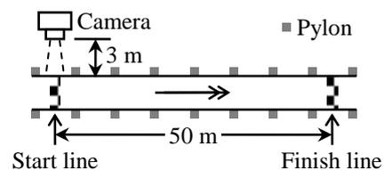
Fig. 2: Drag strip and camera's location
