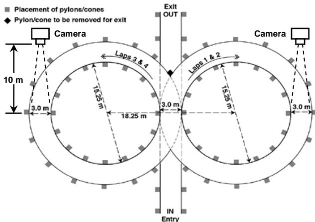
Fig. 4: Skid-pad track and camera location (modified from [10])
