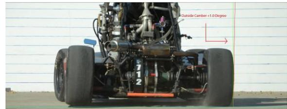
(b)  $-1.0^\circ$ , rear camber =  $+1.00^\circ$ , roll angle =  $0.88^\circ$
