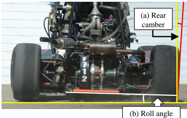
Fig. 5: Measurement of angles
