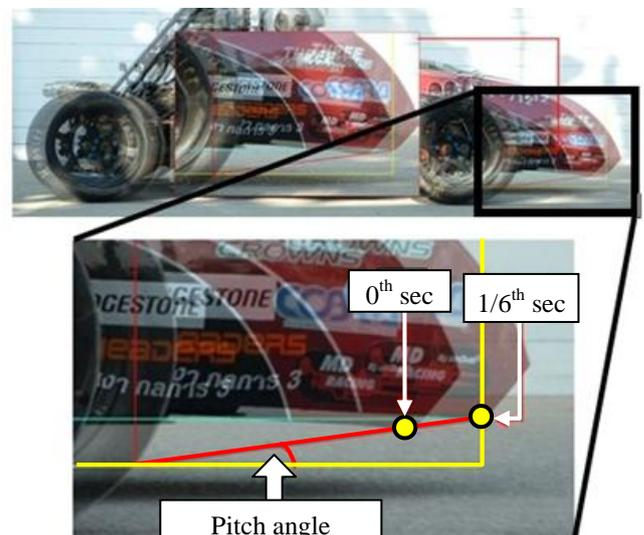
Fig. 3: Measurement of the pitch angle
