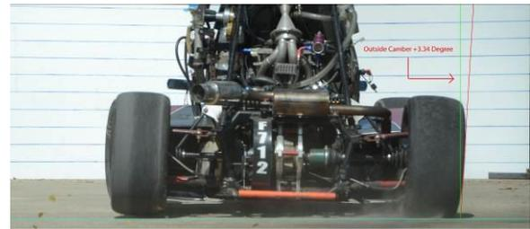
(a)  $0^\circ$ , rear camber =  $+3.34^\circ$ , roll angle =  $1.77^\circ$
