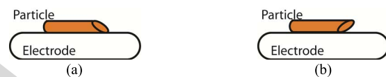
Fig. 2. Orientation of the particle with a sharp end. (a) Tip close to electrode surface. (b) Tip well separated from electrode surface.
