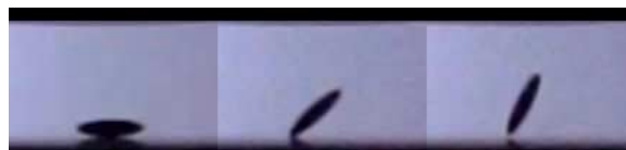
Figure 6. Temporal sequence of the smaller-particle motion (from left to right) when the applied voltage was gradually increased until particle moved.
