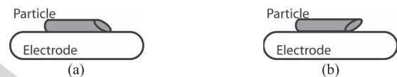
Fig. 2. Orientation of the particle with a sharp end. (a) Tip close to electrode surface. (b) Tip well separated from electrode surface.
