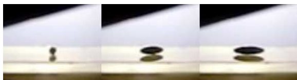
Figure 14. Horizontal rotation of a spheroidal particle on an insulated electrode after electric field application. Images are shown in a temporal sequence from the left hand side.
