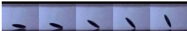
Figure 9. Re-contact of a smaller spheroidal particle after departing from the lower electrode. Particle images are shown in a temporal sequence from left to right.
