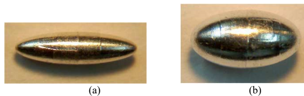
Figure 3. 4-mm long prolate spheroidal particles used in the experiments: (a) smaller particle having 1-mm diameter (minor axis) and (b) larger particle having 2-mm diameter.
