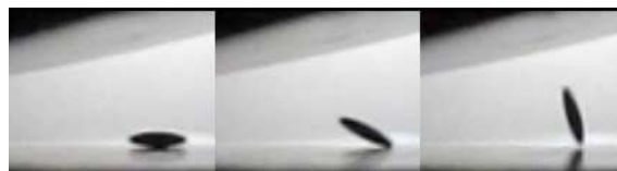
Figure 4. Temporal sequence of vertical rotation from the lying position preceding the particle liftoff.
