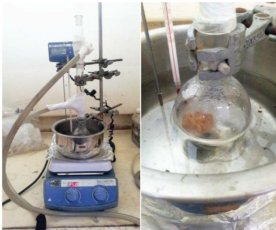
Figure G.1 Picture of reflux set-up for extraction of natural rubber
