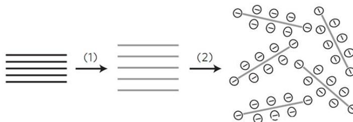
Figure 2.16 Synthesize graphene oxide; (1) Oxidation of graphite using oxidizing agent in strong acid solution; (2) Isolation of graphite layers to graphene oxide sheets 1 .
