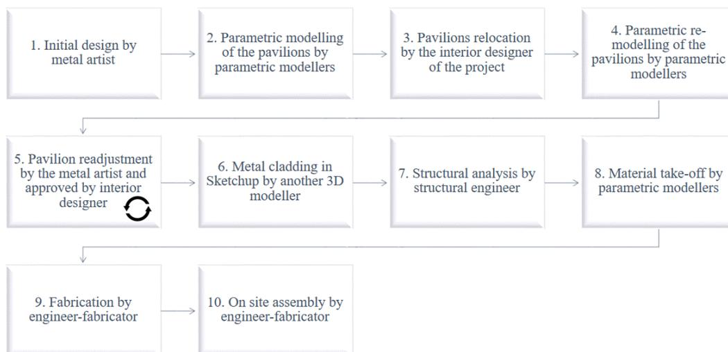
**Figure 1** The design and fabrication process
