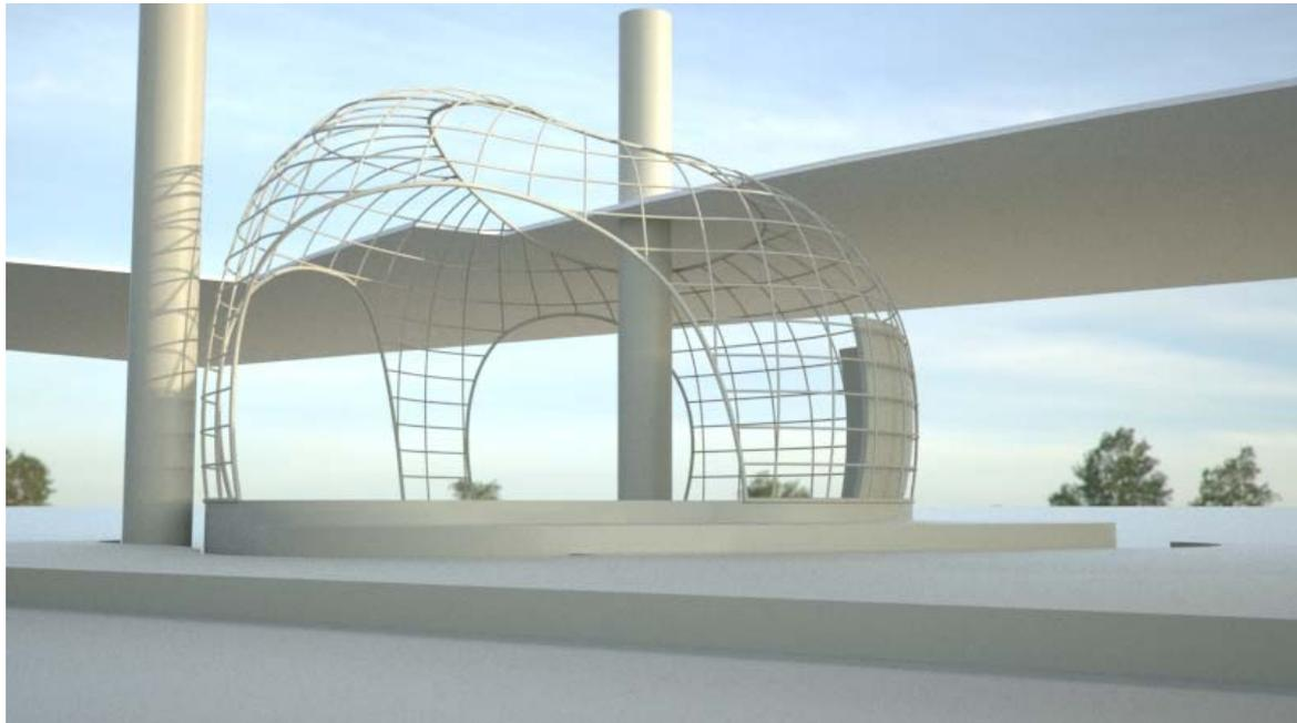
**Figure 6** Pavilion 619/2 was changed from two overlapping pieces to a single piece of structure
