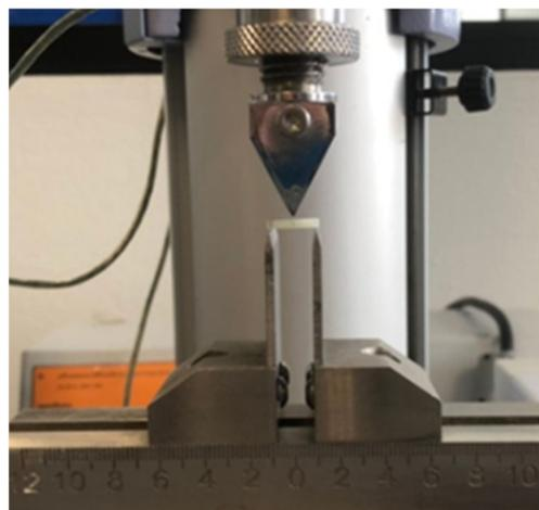
**Figure 2** Picture shown the crosshead is specified for a 50 N axial load at 0.75 mm/min speed until the specimens fractured.
