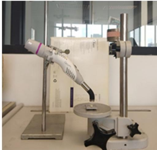
**Figure 1** Picture shown the tip of the curing unit placed at the center of specimens with an angle of 90 degrees.
