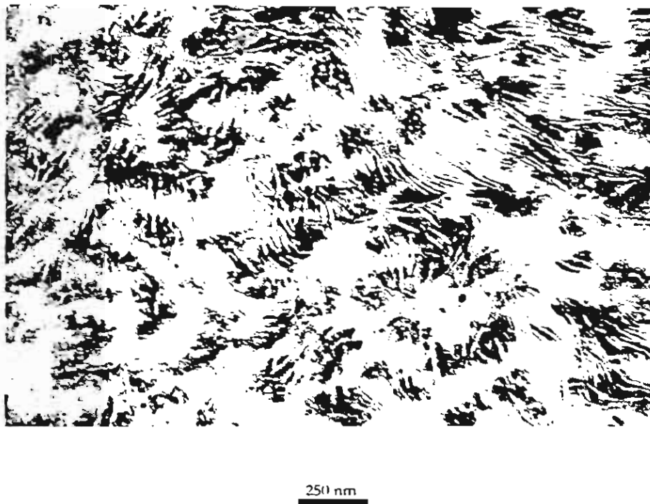
Figure 3.4 TEM micrograph showing the interpenetrating morphology found in the PE1 specimens, molded at 230°C and 0 Pa back pressure, containing 27.9 wt% of EOC2.
