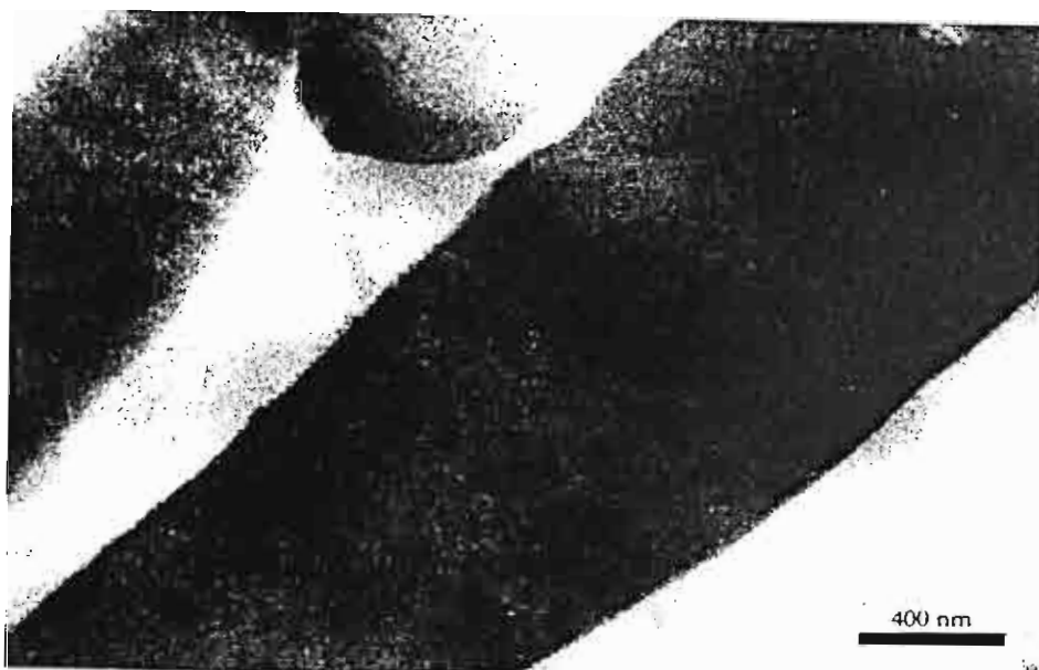
Figure 3. TEM micrograph showing the detail of the morphology of a PP sample containing 40 wt% of EcO 2 . The sample was mixed in an internal mixer, sheared between parallel plates at 230 °C, and then quenched. Micrograph shows a section taken at 5 mm from the center of the sample; at this position, shear rate was 10 s -1 .
