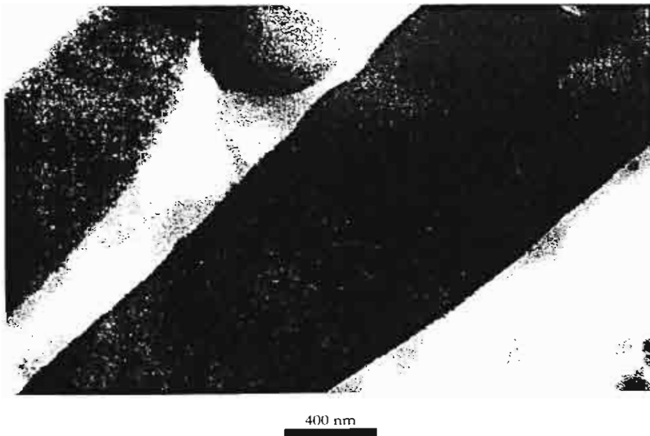
Figure 3.2 TEM micrograph showing the detail of the morphology of a PP sample containing 40 wt% of EOC2. The sample was mixed in an internal mixer, sheared between parallel plates at 230°C, and then quenched. Micrograph shows a section taken at 5 mm from the centre of the sample; at this position, shear rate was 10 \text{s}^{-1} .
