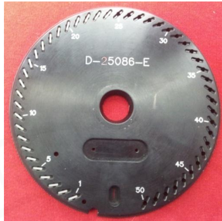
Figure 4.4 Array of thermoluminescence dosimeter (TLD-700) in the TLD planchet.
