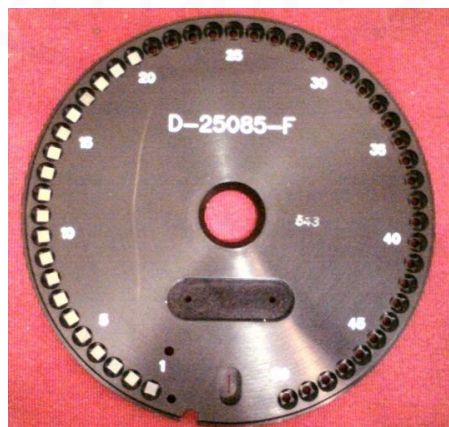
Figure 4.5 Array of thermoluminescence dosimeter (TLD-100H) in the TLD planchet.
