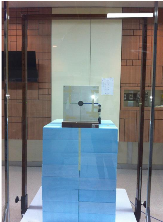
Figure 4.14 Calibration point dose measurement
