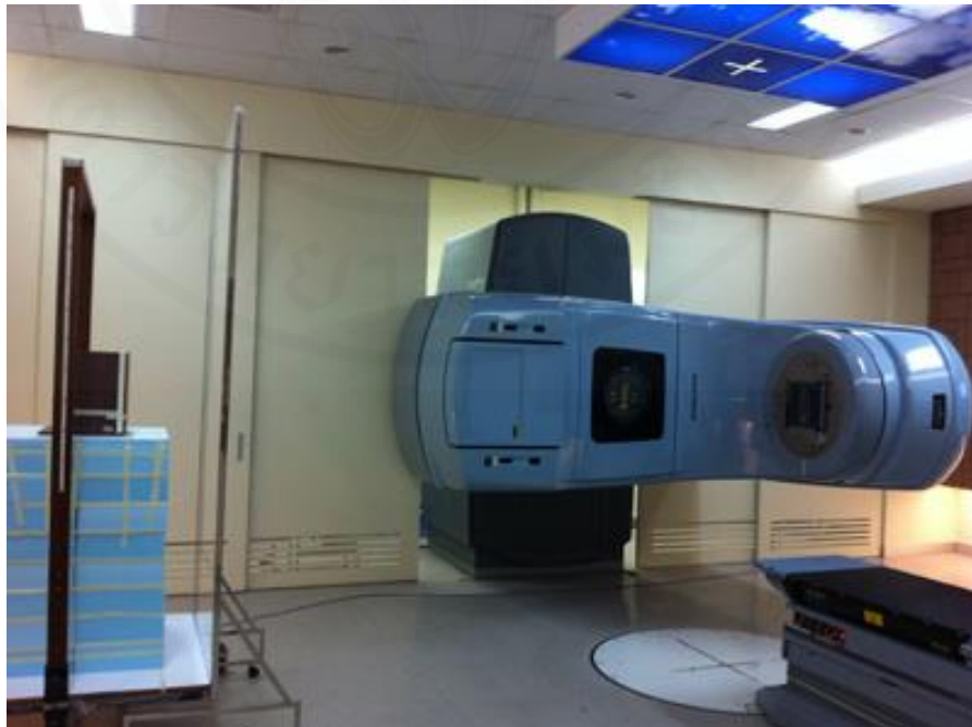
Figure 4.13 Percentage depth dose measurement using Roos chamber.
