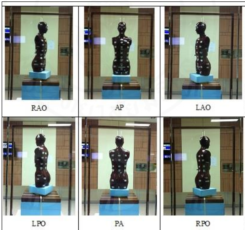
Figure 4.17 Six phantom positions for one complete treatment cycle.
