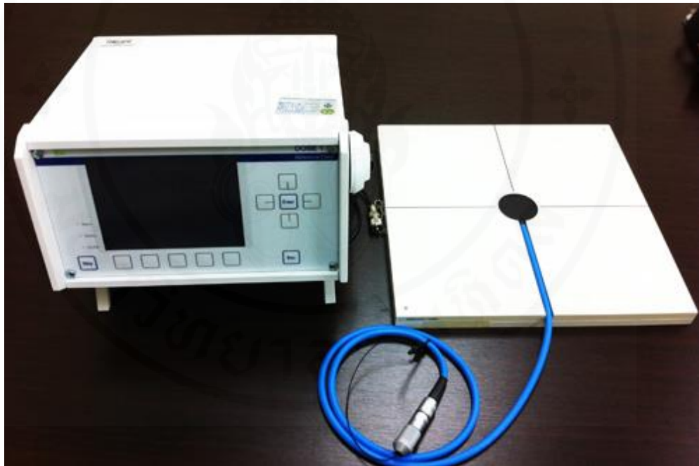
Figure 4.4 Parallel plate Roos chamber and Dose 1 electrometer.
