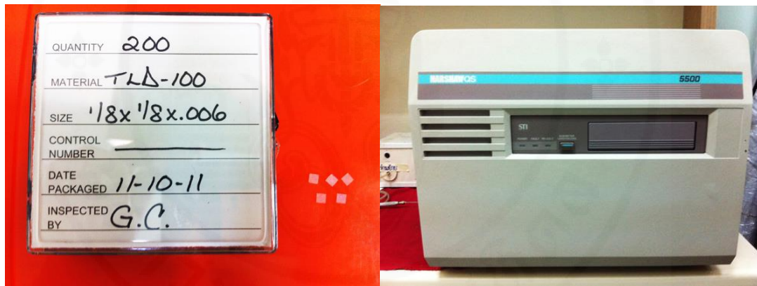
Figure 4.5 TLD- 100 chip and TLD reader system Harshaw 5500.
