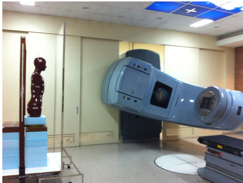
Figure 4.16 Treatment geometry set-up on Rando phantom.
