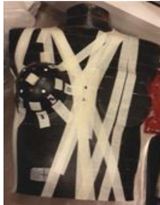
Figure 4.3 The Alderson Rando phantom.
