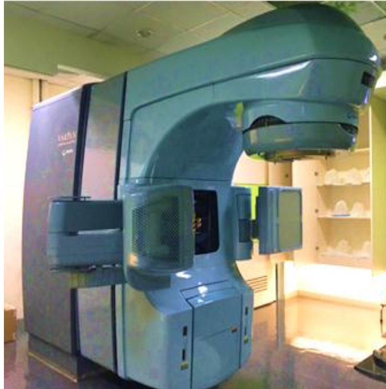
Figure 4.2 Varian Clinac iX linear accelerator
