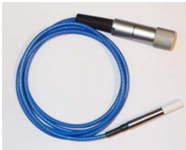
Figure 4.3 The microDiamond detector PTW-60019 (PTW-Freiburg, Germany)
