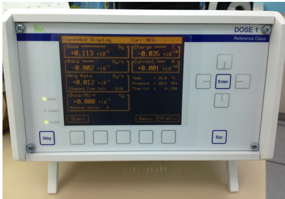
Figure 4.4 DOSE 1: High Performance Reference Class Electrometer.
