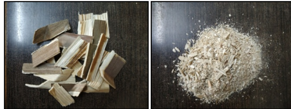
Figure 7: Dry (43seconds grinding time).
