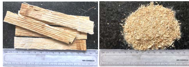
Figure 4: Dry and Compact (40seconds grinding time).
