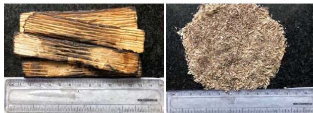
Figure 5: Dry and Torched (33seconds grinding time).
