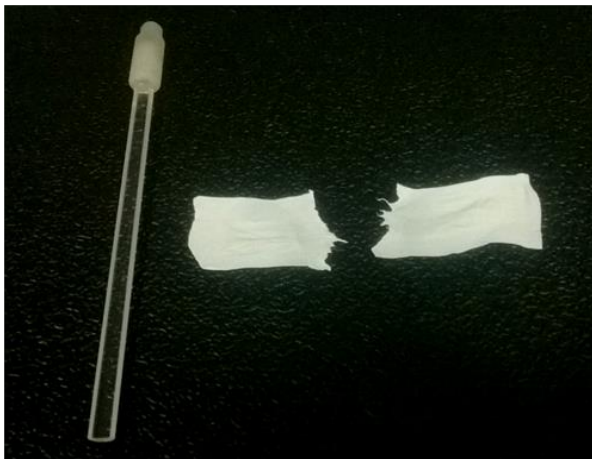
Stretched Teflon tape and the VSM rod
