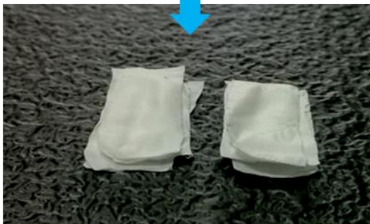
The cut samples ready to be mounted onto the VSM rod
