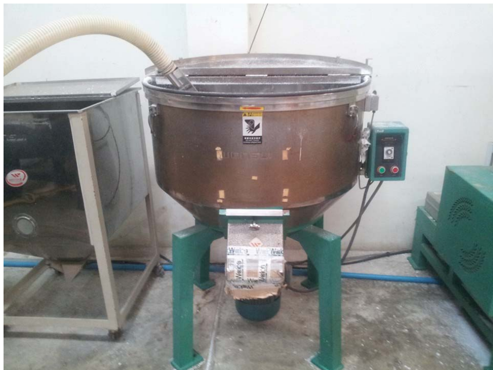
Figure E-2 Gridding machine (15 kW)
