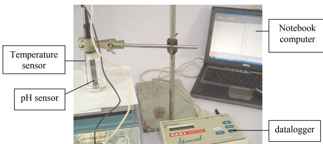
Figure 3.9 A set of equipment for studying the effects of reactant concentrations on the reaction rate
