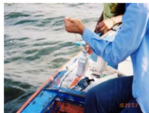
Fig. 3.4 The hydrogen sulfide collecting in the field (a. Pulled the sediment from the PVC, b. Fixed the sediment with Zinc acetate in BOD bottle)
