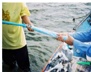
Fig. 3.4 The hydrogen sulfide collecting in the field (a. Pulled the sediment from the PVC, b. Fixed the sediment with Zinc acetate in BOD bottle)
