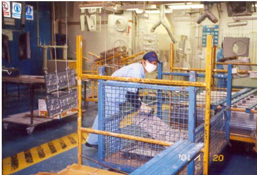
Figure 2-18 The worker brings material to hang them on overhead conveyor.
