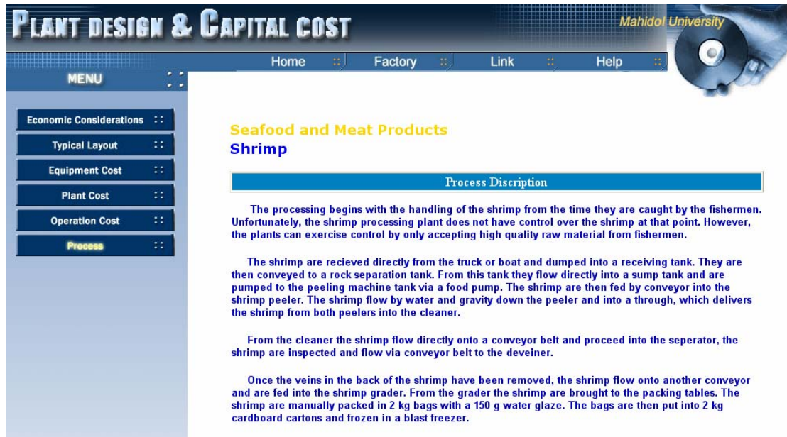
Figure B.15 Screen : Process Description
