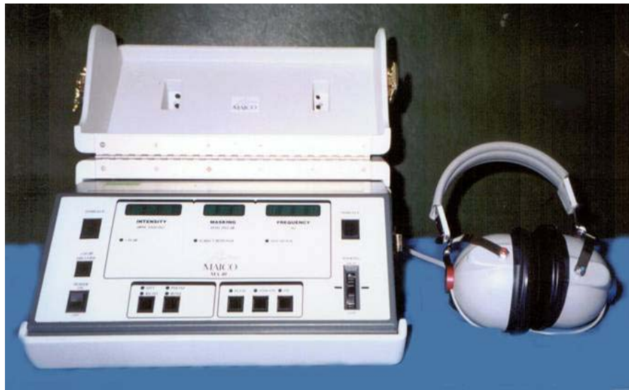
Figure 3.2 Audiometer was used as the sound generator.
