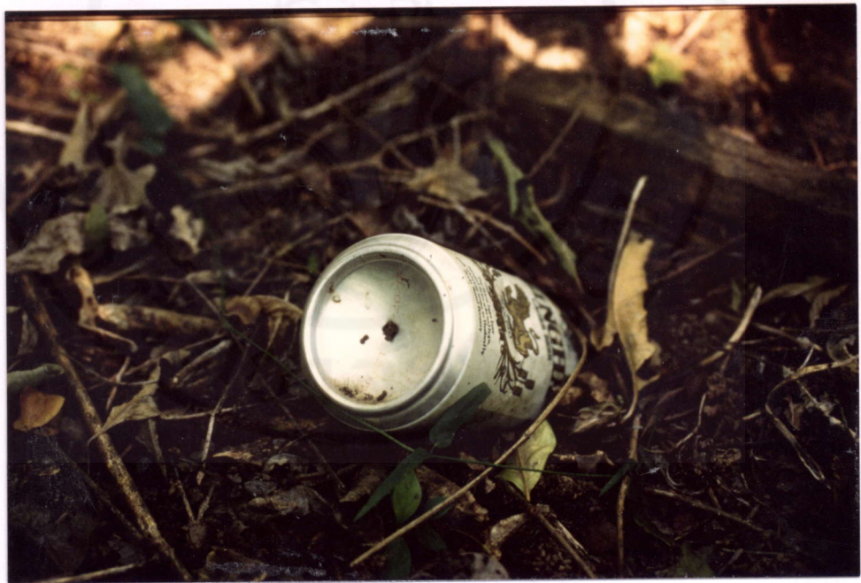
Figure 2.2 Test specimen placed in used-beverage can subjected to macroorganism exposure
