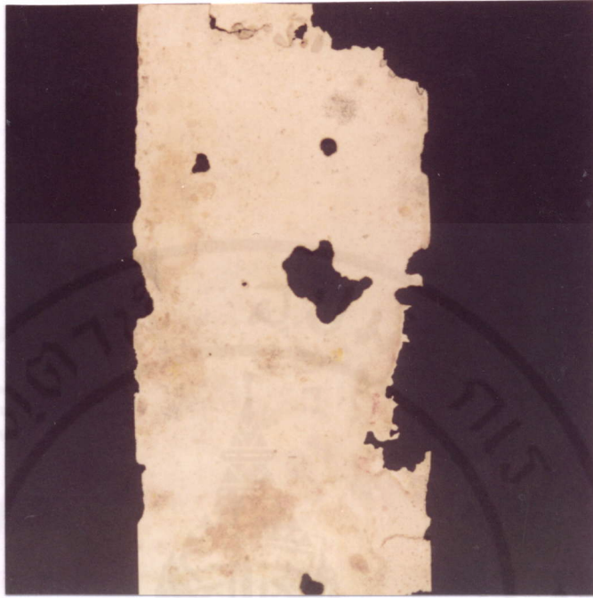
(b) 50% starch content, 224 days exposure, 21.5% weight loss
