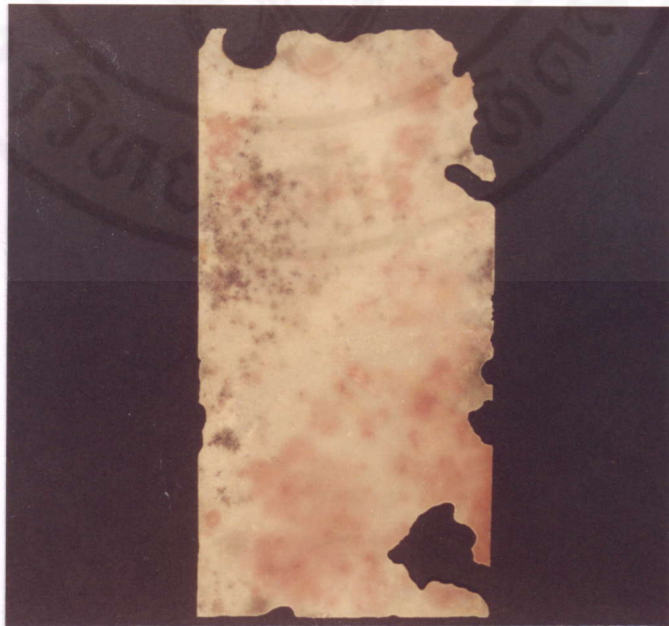
(c) 75% starch content, 175 day exposure, 13% weight loss
