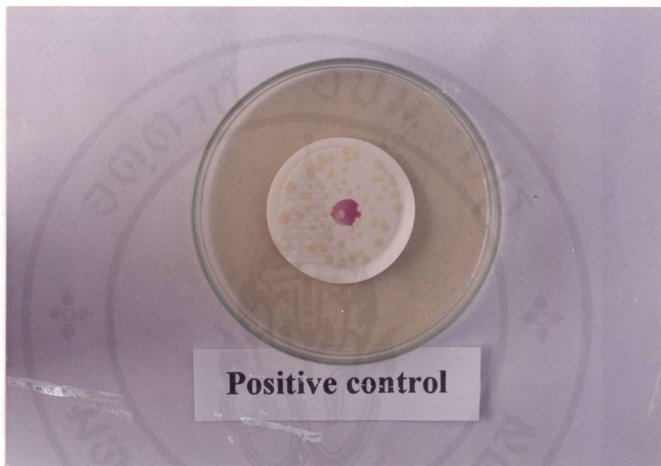
Fig. 29 Photograph of a HA membrane placed over Fluorocult ECD agar plate showing the indole positive with KOVACS' reagent dropped over E. coli colonies. The reagent turns red upon reacted with indole produced by E. coli .
