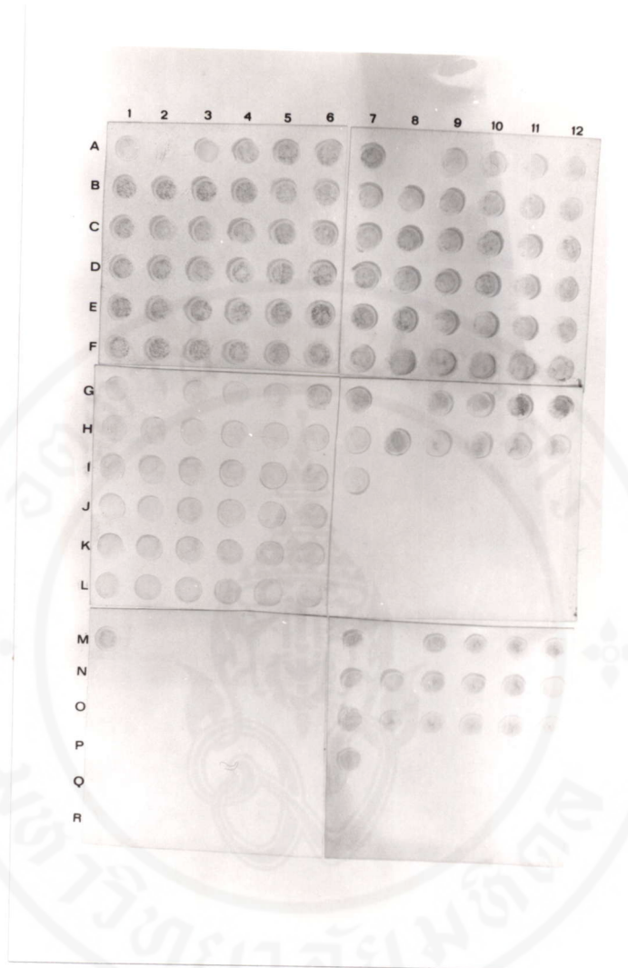
Fig. 15 Dot blot hybridization of E. coli and other bacteria with GA153 probe. All positive signals are E. coli strains except G9-G12, H7-H12 and I7 are Shigella spp. A2, A8, G2, G8, M2 and M8 are Pseudomonas putida . The other negative signal positions are other enteric bacteria or other gram positive bacteria as indicated in Table 5. R8-R12 are blanks.
