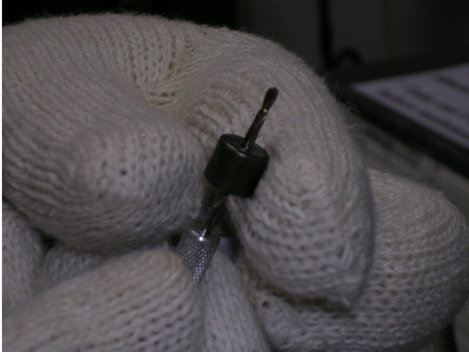
Figure C-8 Hot orifice while cleaning with CC gloves
