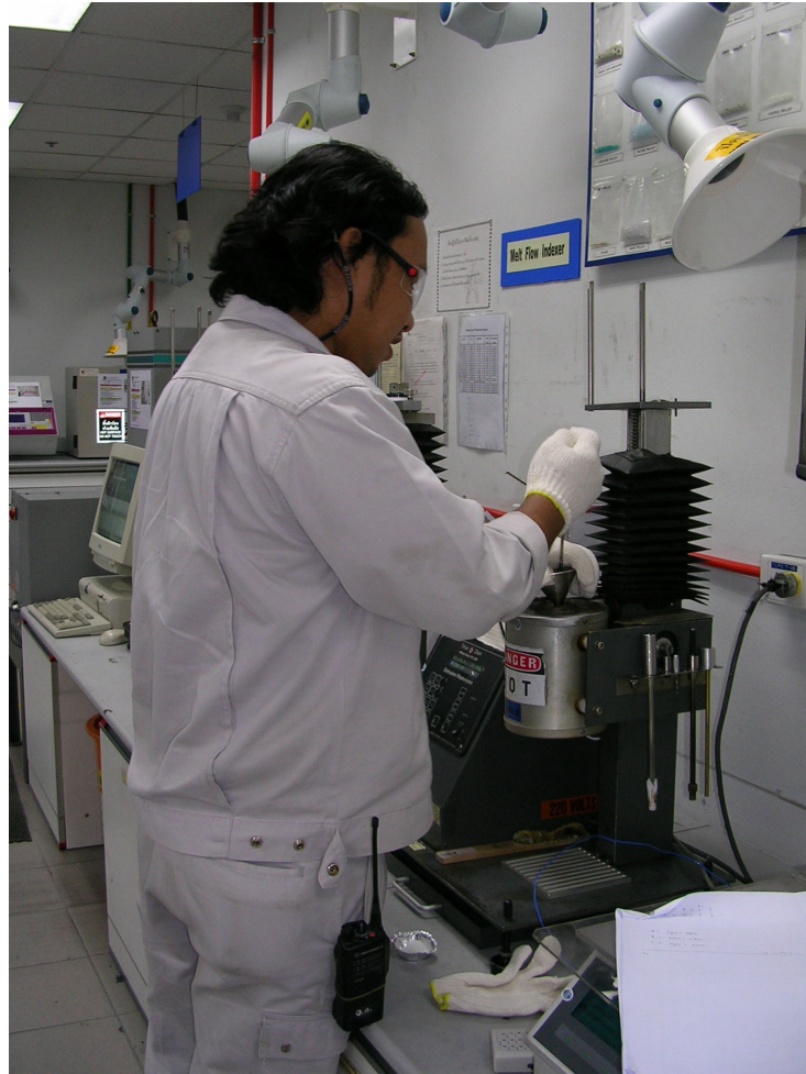
Figure C-4 Melt flow process is being tested by operator
