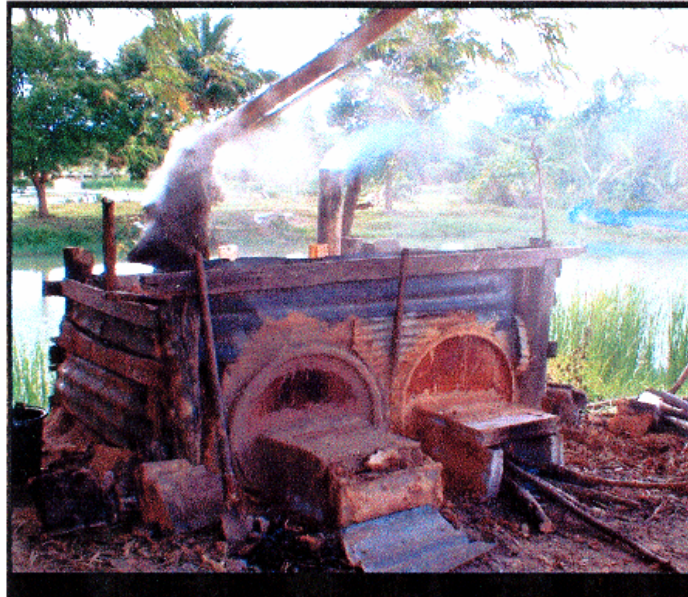
Figure 2.3 High efficiency kiln burning in each step and gathering wood vinegar from burned kiln.
