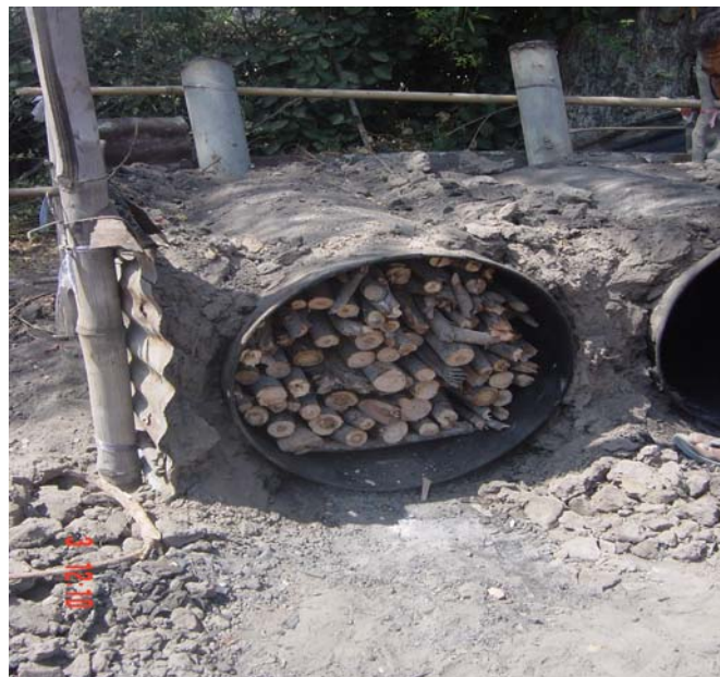
Figure 2.3a Wood arrangement into the kiln
