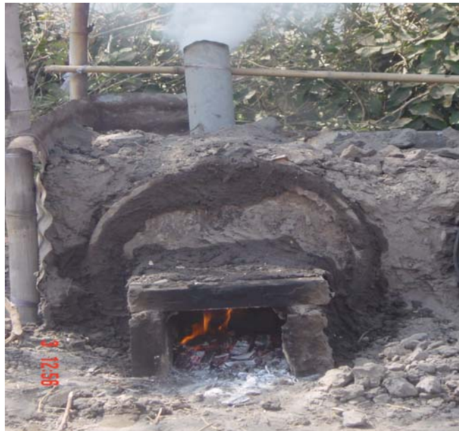
Figure 2.3e Combusting processing of the kiln
