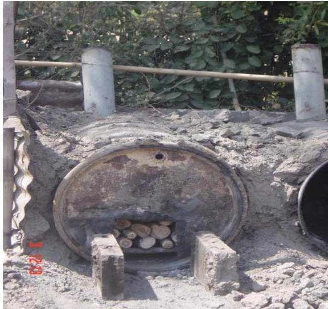
Figure 2.3b Wood arrangement into and ready to close the kiln
