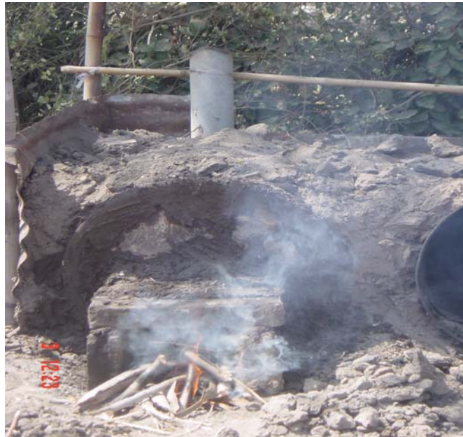
Figure 2.3d Lighting the kiln with fuel
