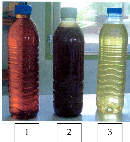
Figure 2.2 showing the variety of wood vinegar from high efficiency kiln burning Bottle 1: Settled wood vinegar Bottle 2: Haven't settled yet Bottle 3: Had distilled already
