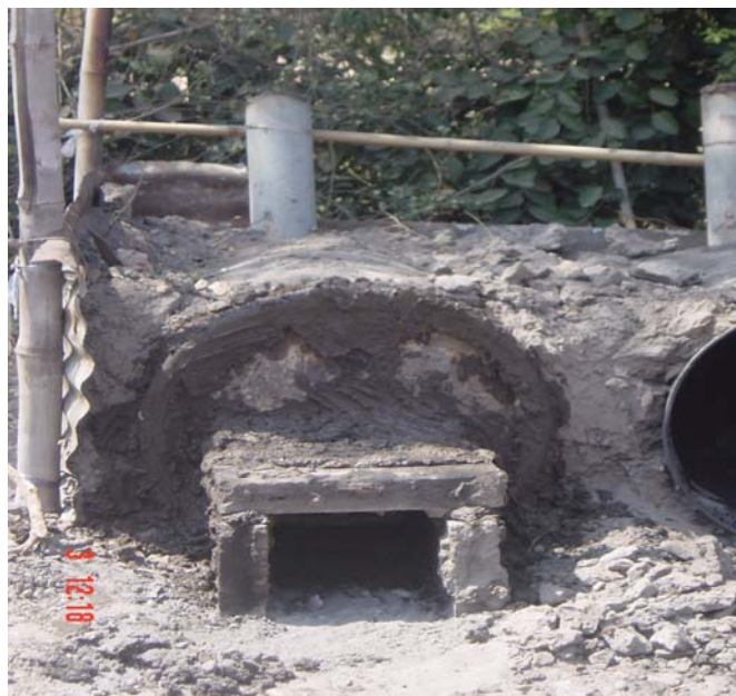
Figure 2.3c Closing the air passage of the kiln with mud soil
