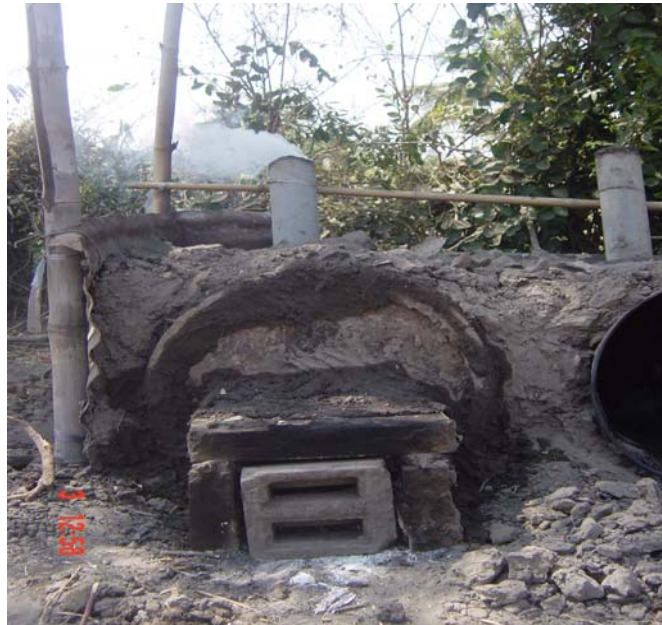
Figure 2.3f Closing air passage for controlling the air in order to complete burning
