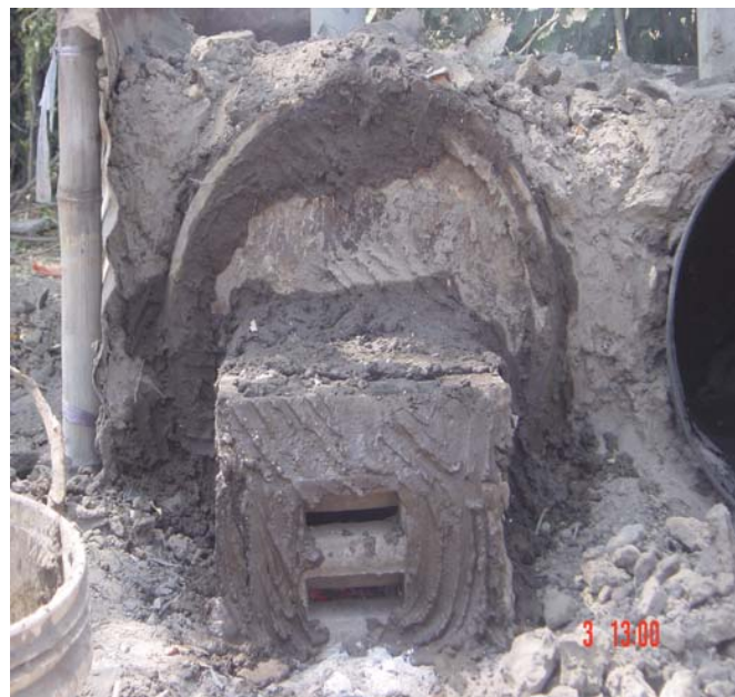
Figure 2.3g closing the kiln in order to decrease temperature in the kiln
