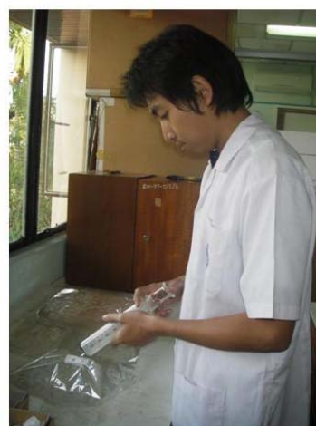
2. Inject the stock odorant air sample into the odor bag, volume 3 liters
