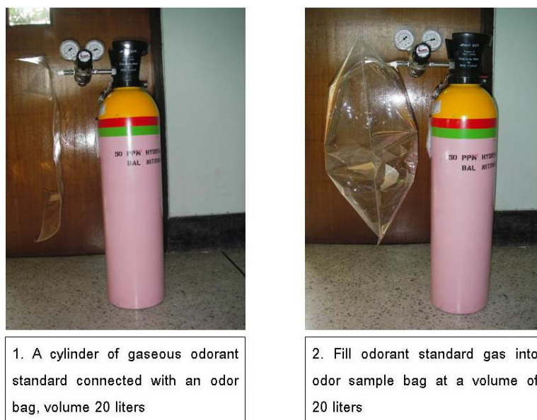
Figure 3-9: Transfer of gaseous odorant standard into an odor sample bag
