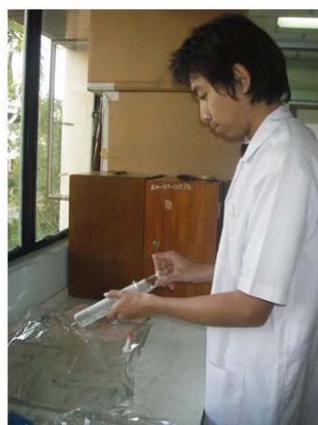
1. Withdraw the stock odorant air sample from the odor bag, volume 20 liters
