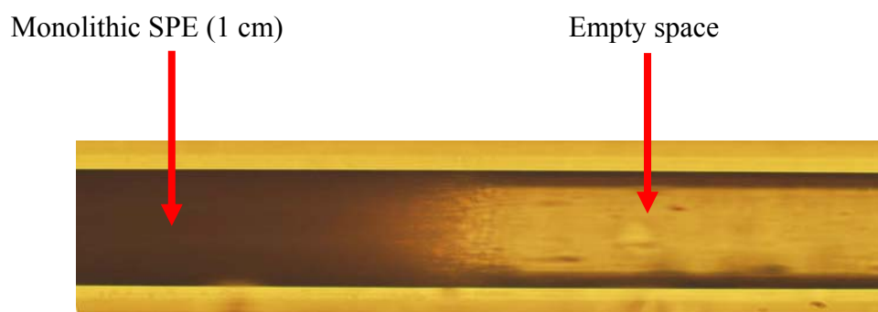
Figure 4.7 Microscopic picture of the in-line monolithic SPE-CE capillary.
