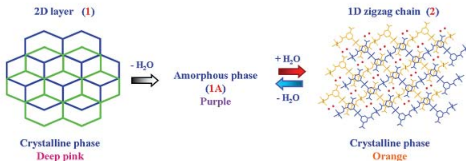
Figure 67 Schematic diagram illustrates the structural conversion of 2D layer to 1D chain structures by thermal dehydration and rehydration processes.
