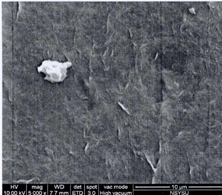
Figure 4.19 SEM photographs of membrane surface at the first stage (Non-dosed).
