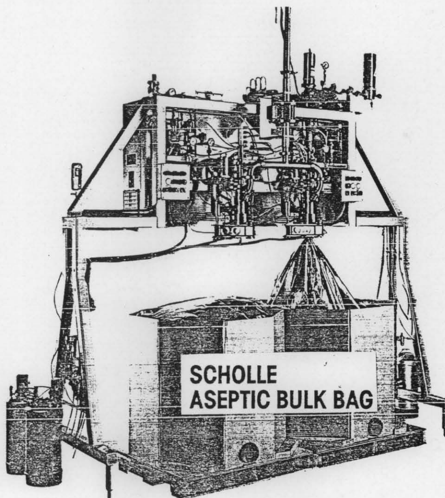
Auto-Fill 10-2E with expanded frame shown filling 220 gallon aseptic bags in corrugated bins
