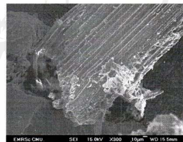
Fig. 5 SEM micrographs for untreated bamboo fiber reinforced epoxy composite fracture after tensile loading.
