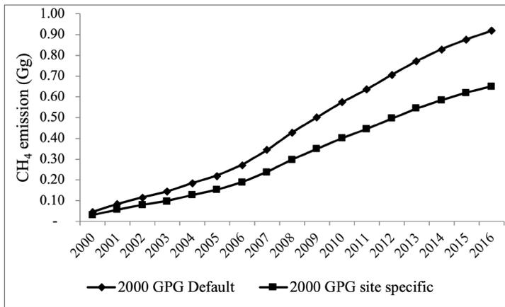
Figure 4. Methane emission estimated by 2000 GPG approach comparing between default and site specific emission factors
