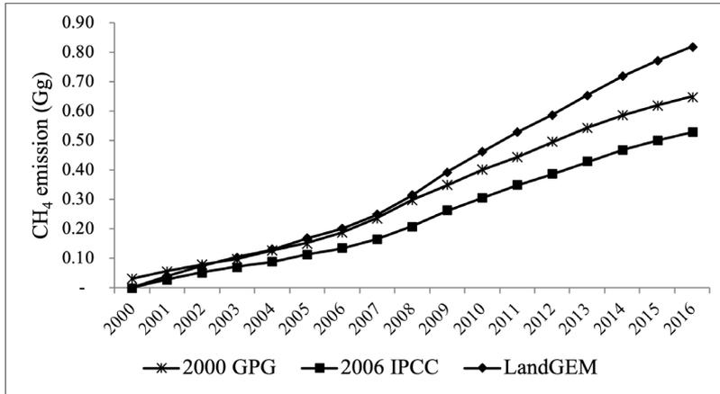
Figure 8. Comparison of estimated methane emission by different approaches using site specific emission factors
