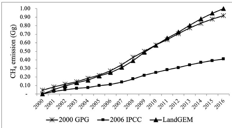
Figure 7. Comparison of estimated methane emission by different approaches using default values
