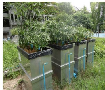
Figure 1. Constructed wetland systems planted with umbrella sedge ( Cyperus involucratus Rottb)
