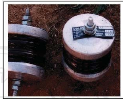
รูป 16-1 Spark gap lightning arrestors
