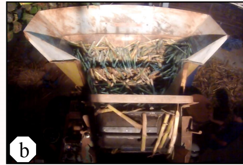
Fig. 5 Sample of recorded frame during the stationary test of a) the original metering device and b) the developed metering device
