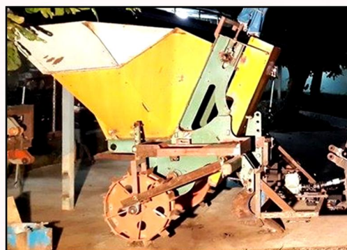
Fig. 1 The modified billet planter Austoft 750 BP that used for the experiment
