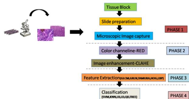
Figure 1. The block diagram
