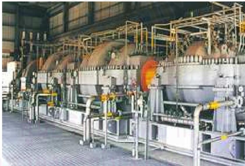
Figure 3.4 Cracked gas compressor
