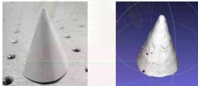
**Figure C-4:** Real object and reconstructed 3D models of cone
