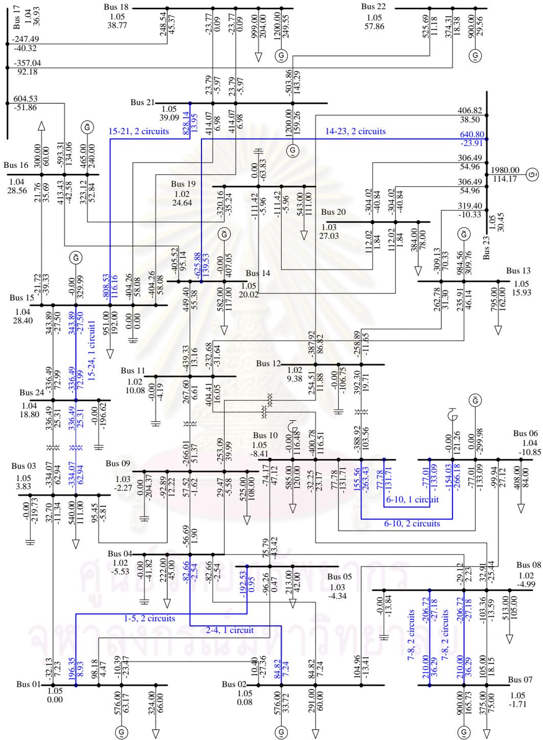
Figure 6.11 Power flow diagram of the first stage for IEEE-24 bus system
