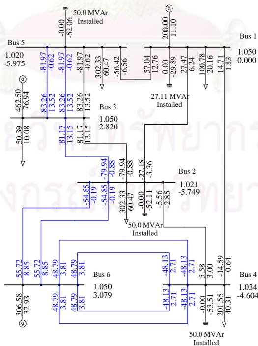
Figure 6.6 Power flow diagram of the second stage for Garver system
