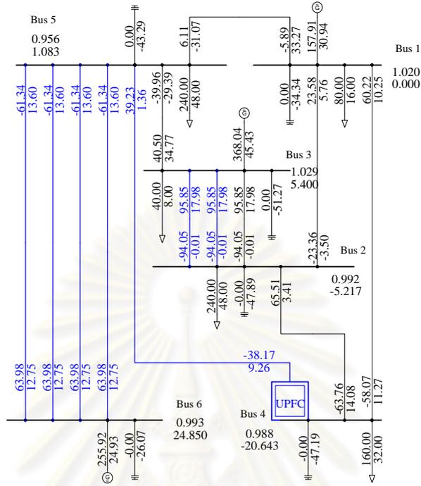
Figure 6.20 Power flow diagram with installed UPFC
