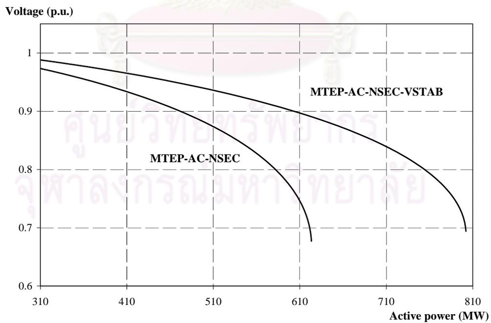
Figure 6.18 V-P curve of the second stage at bus 2
