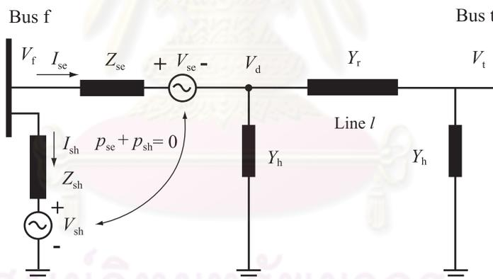
Figure 5.2 Equivalent circuit of UPFC
