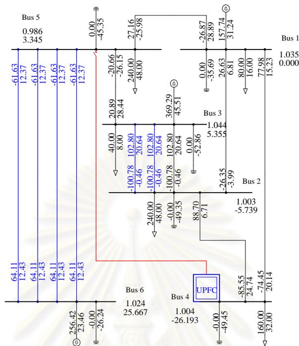
Figure 6.22 Power flow diagram with line 4–5 tripped
