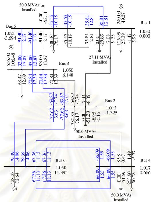
Figure 6.7 Power flow diagram of the third stage for Garver system
