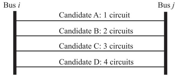
Figure 3.2 Example of candidate branch definition
