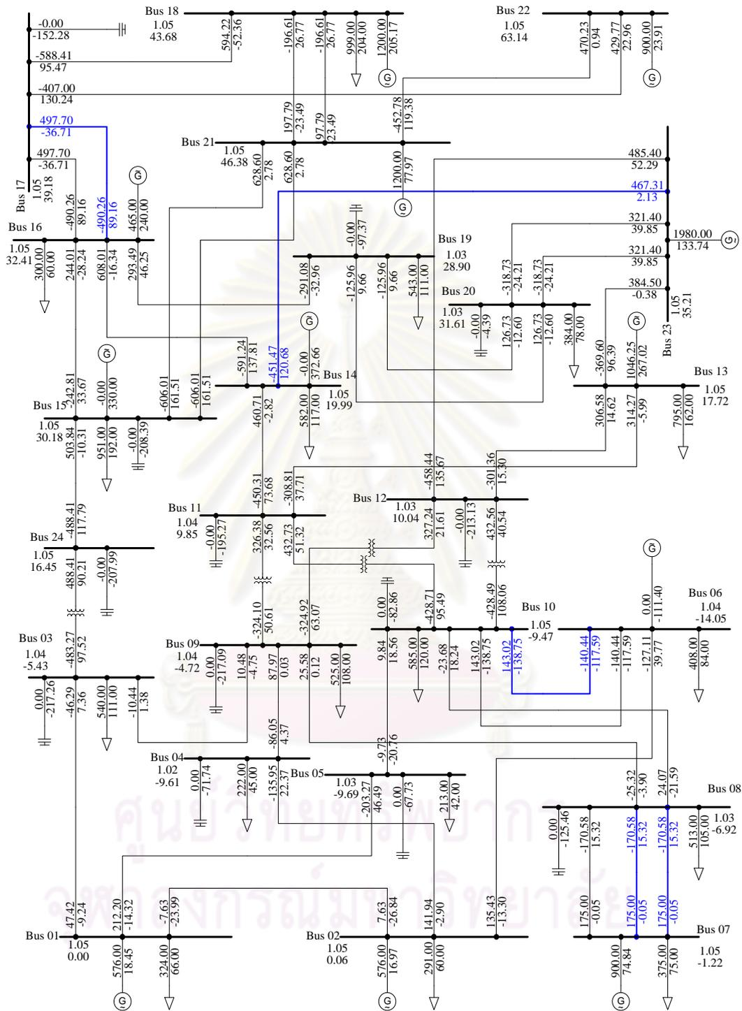
Figure 6.4 Power flow diagram of STEP-AC problem for IEEE-24 bus system
