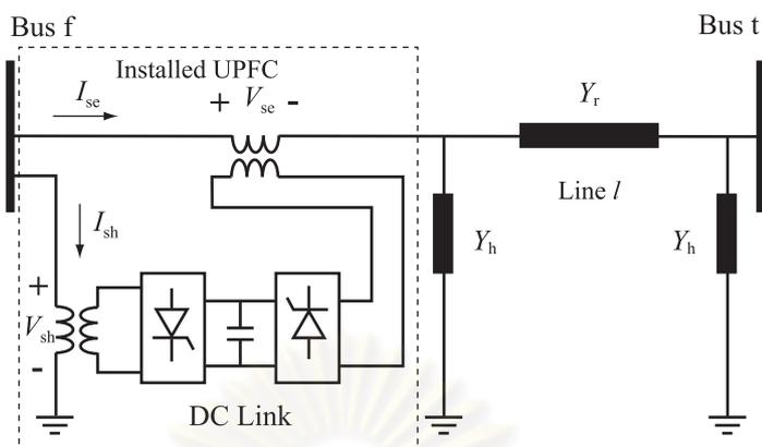
Figure 5.1 Operating diagram of UPFC
