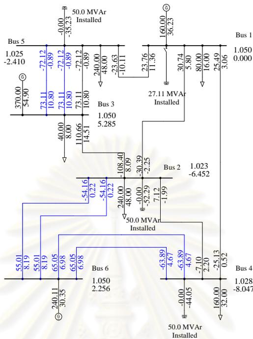
Figure 6.5 Power flow diagram of the first stage for Garver system
