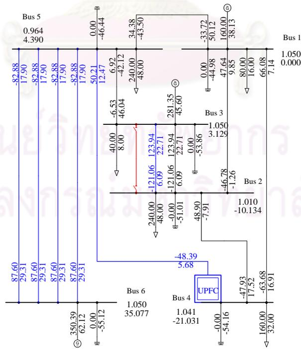
Figure 6.21 Power flow diagram with line 2-3 tripped
