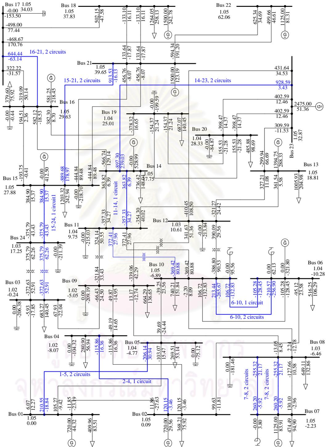
Figure 6.13 Power flow diagram of the third stage for IEEE-24 bus system
