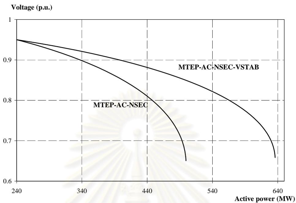
Figure 6.17 V-P curve of the first stage at bus 2
