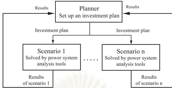
Figure 2.1 Conventional method for solving TEP
