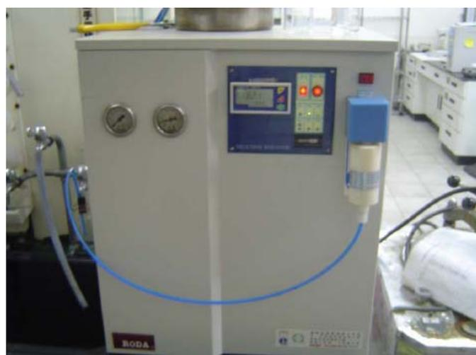
Figure B.9. Demineralization Water Production Instrument
