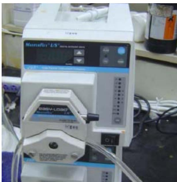
Figure B.13. Hydrogen Peroxide Feeding Pump Instrument
