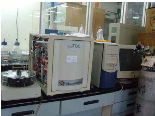
Figure B.7. Total Organic Carbon (TOC) Analyzer Instrument
