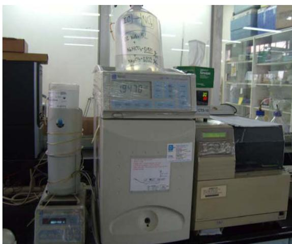
Figure B.8. Liquid Ion Chromatography (IC) Instrument
