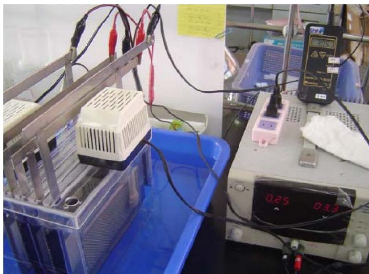
Figure B.2. Electro-Fenton reactor setup
