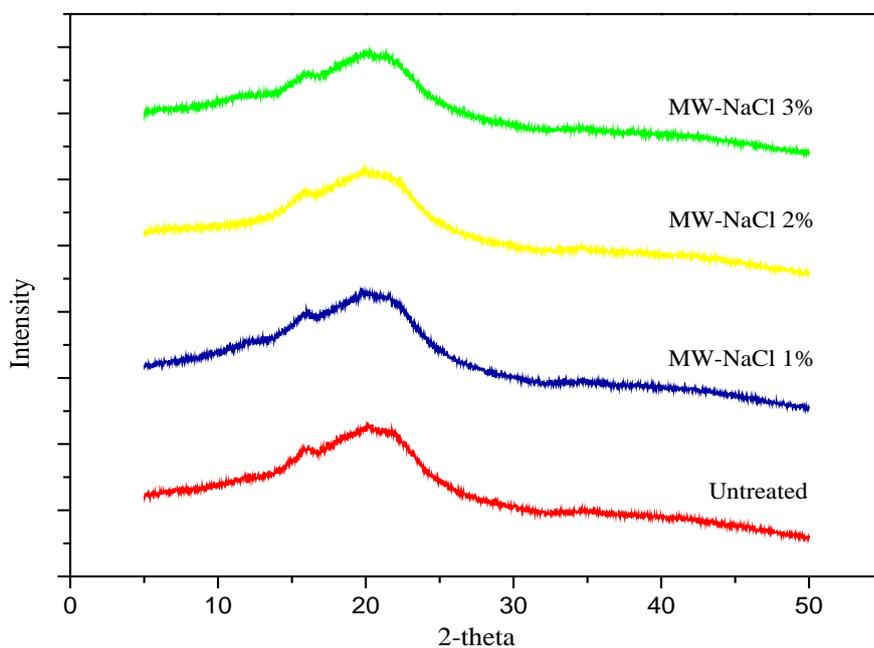
Figure 3 X-Ray diffraction of untreated and treated SCGs.
