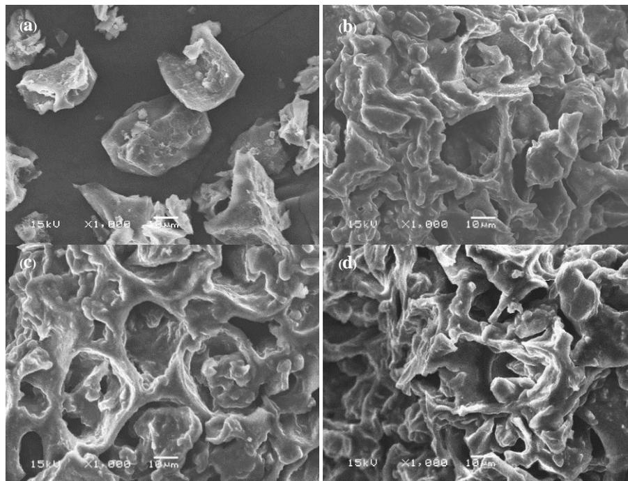
**Figure 1** SEM of (a) untreated (b) 300 W, 1% for 3 min (c) 300 W, 2% for 3 min and (d) 300 W, 3% for 3 min.
