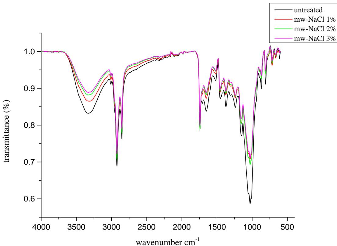
Figure 2 FTIR spectra of SCGs by using microwave-NaCl pretreatment
