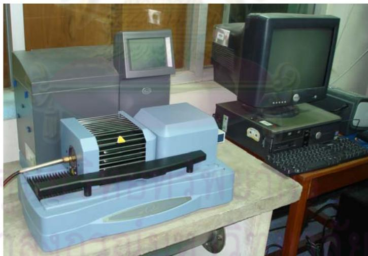
**Figure 4.12:** Thermogravimetric analyzer.
