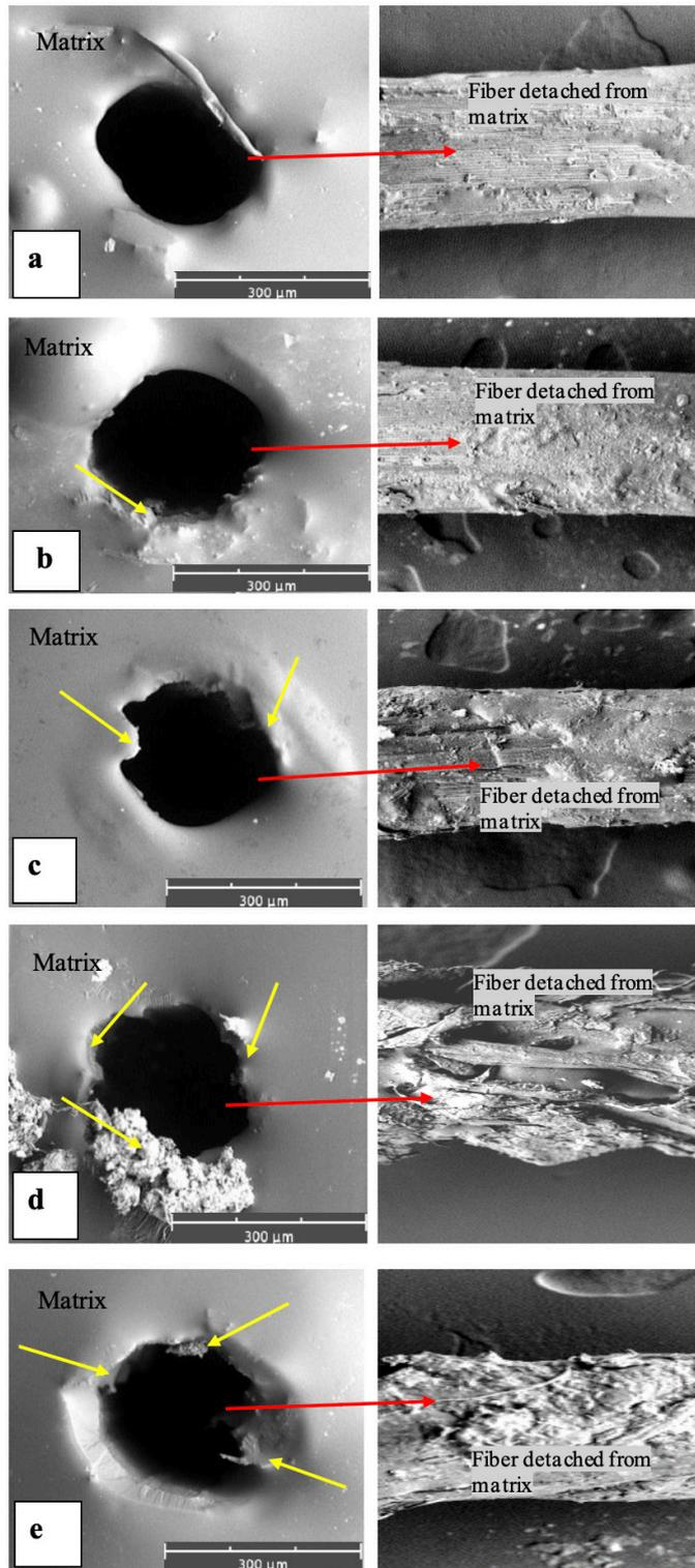
Figure 8. KSEM pull-out tests: (a). WF, (b). F5H, (c). F10H, (d). F15H, (e). F20H
