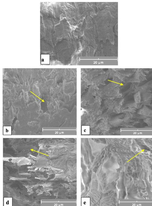
**Figure 7.** KPLF cross-section SEM result, (a).WT, (b).F5H, (c).F10H, (d).F15H, (e).F20H
