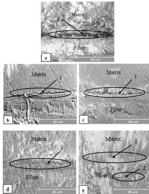
**Figure 6.** SEM for the KPLF interface interlocking with epoxy matrix(a). WT, (b).F5H, (c).F10H, (d).F15H, (e).F20H
