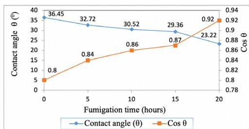
Figure 4. KPLF fumigation time toward the contact angle size and Cos epoxy matrix droplet
