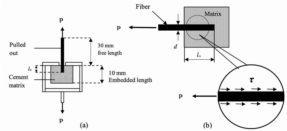
**Figure 2.** Pull-out test mechanism (a).Single fiber pull-out specimen (b).Interfacial strain and shear balance between the fiber surface and epoxy matrix (Palungan, 2016)
