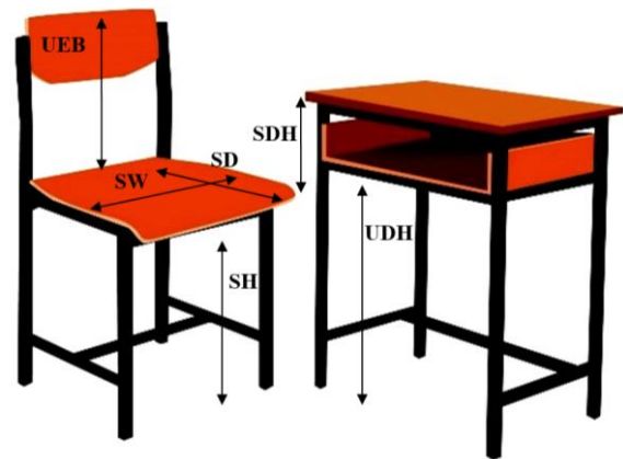
Figure 2. School furniture dimensions; UEB=upper edge of backrest; SW=seat width; SD=seat depth; SH=seat height; SDH=seat to desk height; UDH=underneath desk height.
