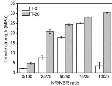
Figure 4. Tensile strength of the uncoated NR/NBR blends (T-0) and 20 wt% treated distillate aromatic extract oil-coated sulfur (T-20).
