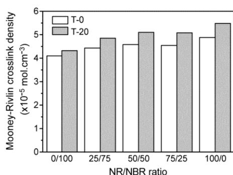
Figure 7. Mooney-Rivlin crosslink density of the uncoated NR/NBR blends (T-0) and 20 wt% treated distillate aromatic extract oil-coated sulfur (T-20).
