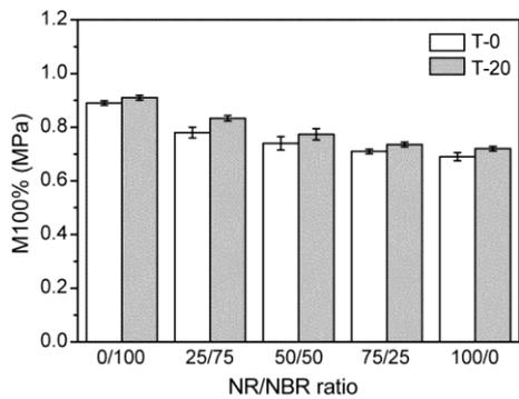
Figure 3. Tensile modulus ( $M_{100}$ ) of the uncoated NR/NBR blends (T-0) and 20 wt% treated distillate aromatic extract oil-coated sulfur (T-20).
