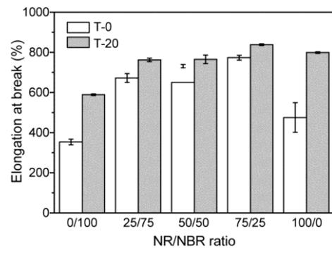
Figure 5. Elongation at break of the uncoated NR/NBR blends (T-0) and 20 wt% treated distillate aromatic extract oil-coated sulfur (T-20).
