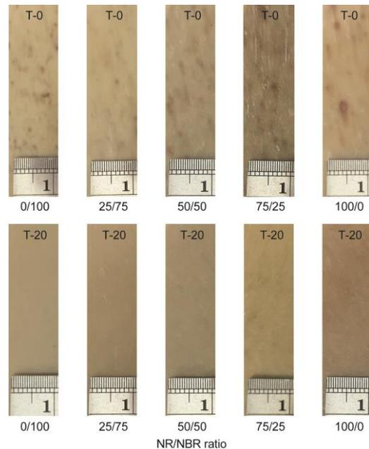
Figure 6. Photographs of the uncoated NR/NBR blends (T-0) and 20 wt% treated distillate aromatic extract oil-coated sulfur (T-20). Scale = centimeter.
