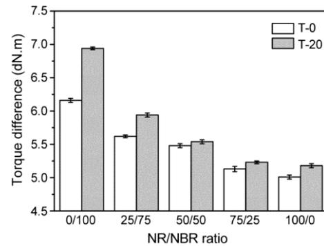
Figure 1. Torque difference of the uncoated NR/NBR blends (T-0) and 20 wt% treated distillate aromatic extract oil-coated sulfur (T-20).
