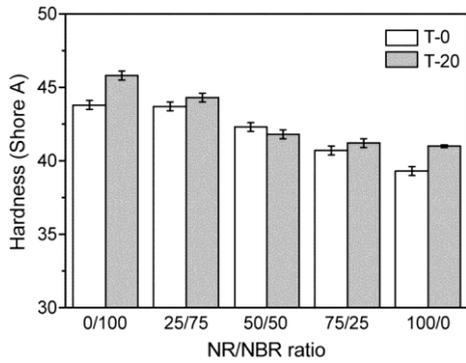
Figure 2. Hardness of the uncoated NR/NBR blends (T-0) and 20 wt% treated distillate aromatic extract oil-coated sulfur (T-20).
