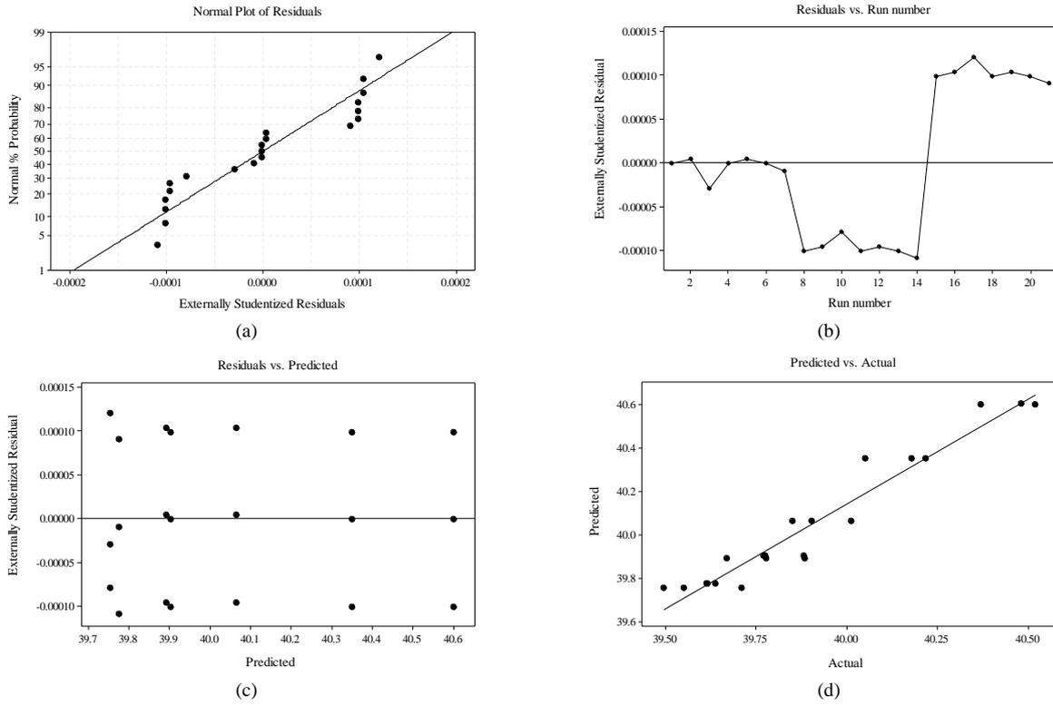
Figure 2. Reliability and validity tests of the regression model for, as an example, total solids (TS): (a) the probability of residuals, (b) the model residuals associated with the 21 experimental runs, (c) the residuals relative to the predicted TS, (d) the observed vs. the predicted TS values.
