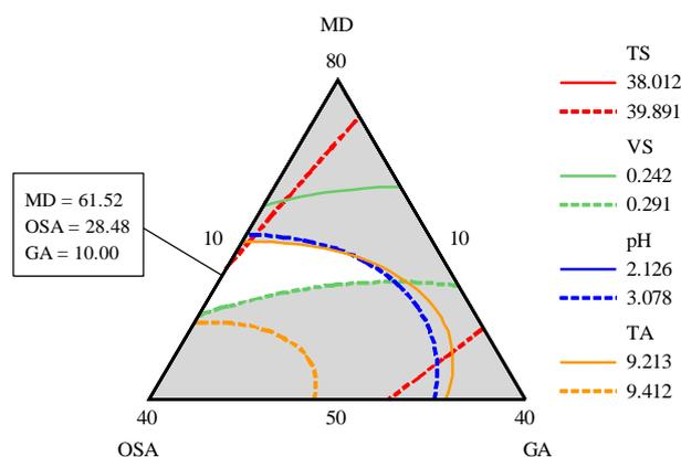
Figure 4. The optimal region of the carrier-mixture concentrations with four physicochemical attributes (TS, VS, pH, TA) of the final tamarind powder closely resembling the fresh tamarind pulp, where MD, OSA, GA denote maltodextrin, octenyl succinic anhydride, and gum arabic, respectively.
