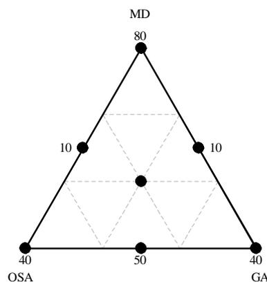
Figure 1. The experimental three-factor simplex lattice mixture design, where MD, OSA, and GA respectively denote maltodextrin, octenyl succinyl anhydride, and gum arabic.
