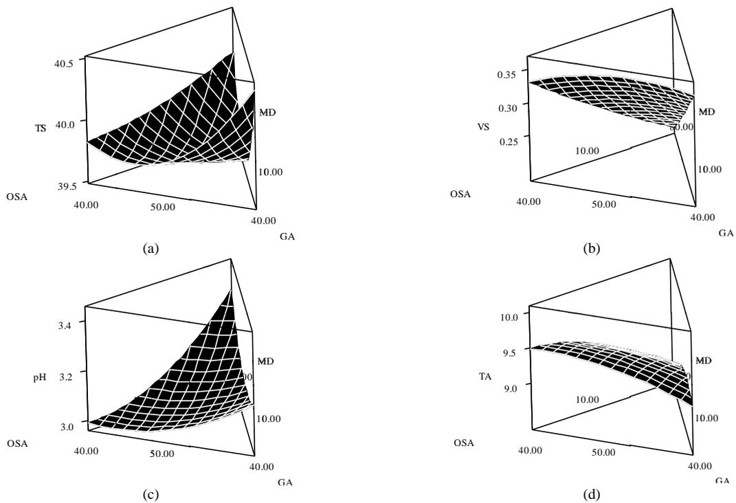
Figure 3. Response surface plots of the physicochemical characteristics of the drum-dried tamarind powders relative to the MD-OSA-GA mixture concentrations: (a) total solids (TS), (b) viscosity (VS), (c) pH values (pH), and (d) total acidity (TA).
