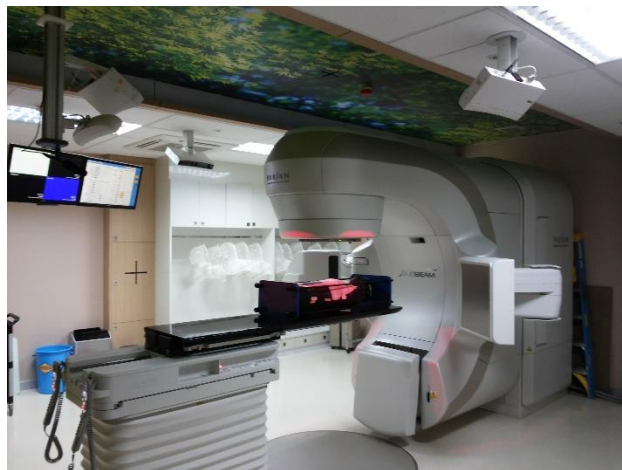
Figure 3.8 The AlignRT system installed in TrueBeam linear accelerator
