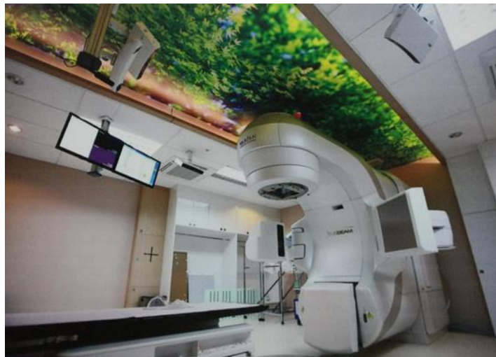
Figure 4.1 Linear Accelerator: TrueBeam with 3D on-board CT and 3D surface tracking system.
