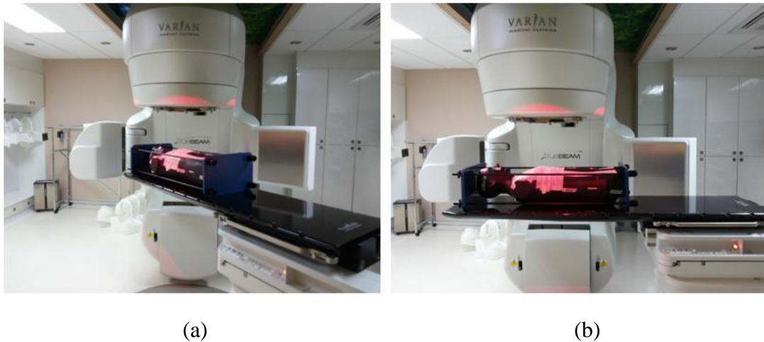
Figure 4.12 The phantom setting up for couch angle effect test at (a) 135 and (b) 270 degree couch angle.
