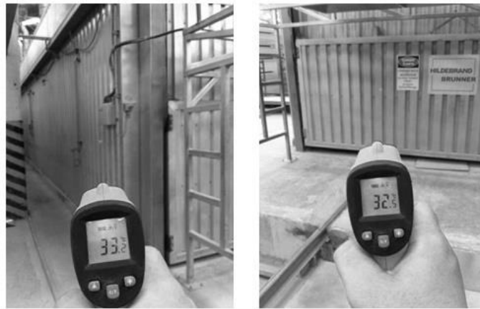
Figure 4.5 Temperature at dryer surface
