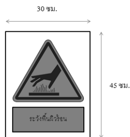
Figure 4.17 Warning sign at surfaces of material, equipment with higher than 60 °C
