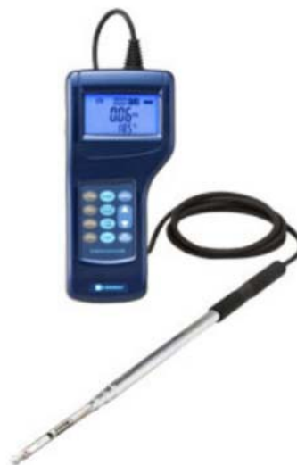
Figure A-2 Kanomax Anemomaster Standard Model 6035 Multi-function thermal anemometer
